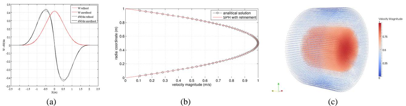
Fig 1: the kernel and kernel gradient approximation for an unsplit particle (unrefined) and its daughter particles arrangement (refined) (a); Poseuille flow, velocity profile (b) and particle distribution in 3D (c)
